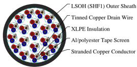
Tinned Copper Drain Wire XLPE Insulation Al/polyester Tape Screen
